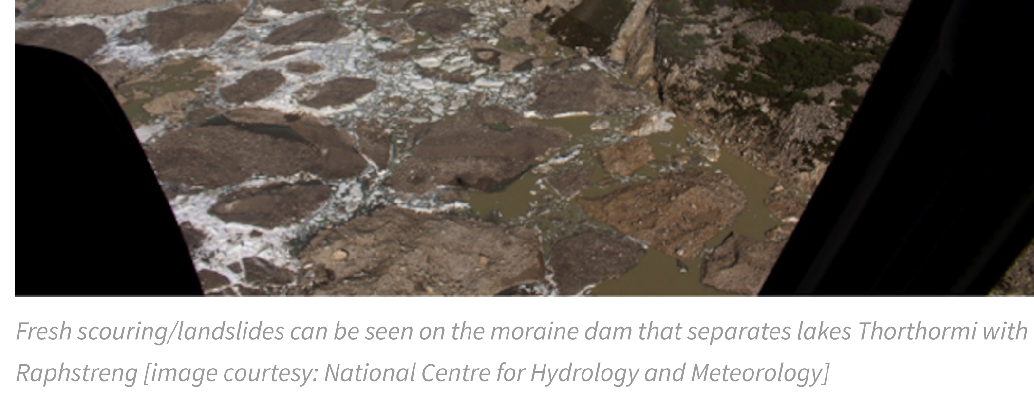
Fresh scouring/landslides can be seen on the moraine dam that separates lakes Thorthormi with Raphstreng [image courtesy: National Centre for Hydrology and Meteorology]
